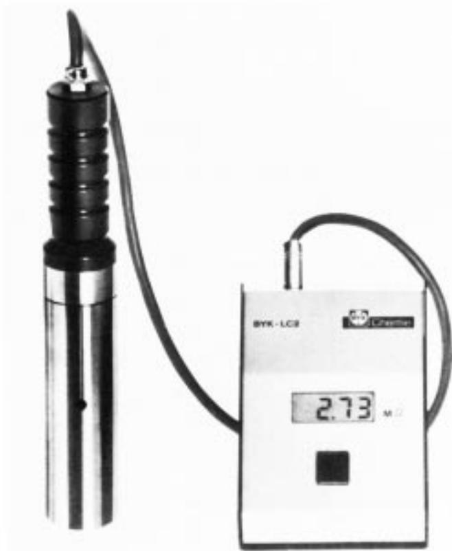
**FIG. 2 Conductivity Meter**
